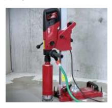
Use tool equipped with integrated water delivery system None that supplies water to cutting surface
